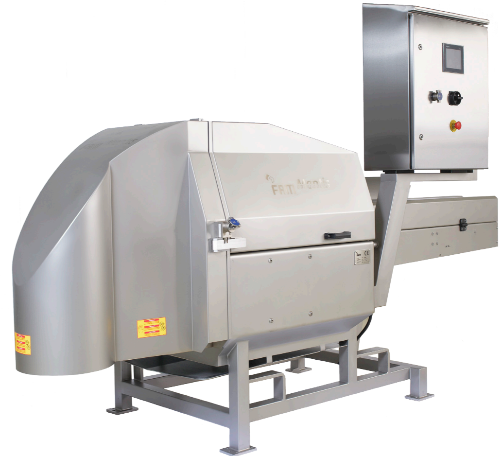
Highly versatile V-belt transverse slicer
